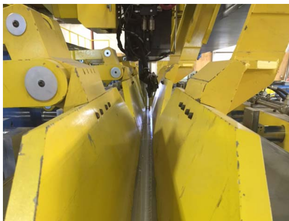
FIGURE 6: Top Plate Friction Stir Welding
