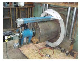
approximately three to four days to rough cut the shaft, approximately one day to polish the shaft, and approximately half a day to machine the transition radius. Two trunnion shafts were machined at a time with continuous shifts working 24 hours a day. Each shaft averaged between 5 and 6 days to complete all machining efforts.
