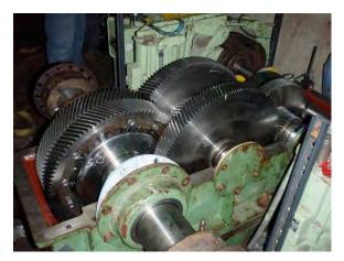
Based on the successful performance of the temporary repairs within the northwest leaf, it was determined to install the new parts in the differentials on the northeast and southwest leafs, and to perform a temporary repair on the southeast leaf. This work was completed within the scheduled six week closure and reduced speed operation of all leafs was restored.
