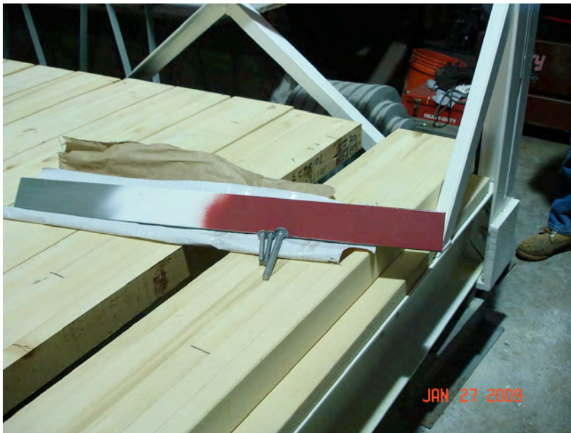
FIGURE 18: Paint sample for approved three coat system. Note rehabilitated sheave assembly in the background.
