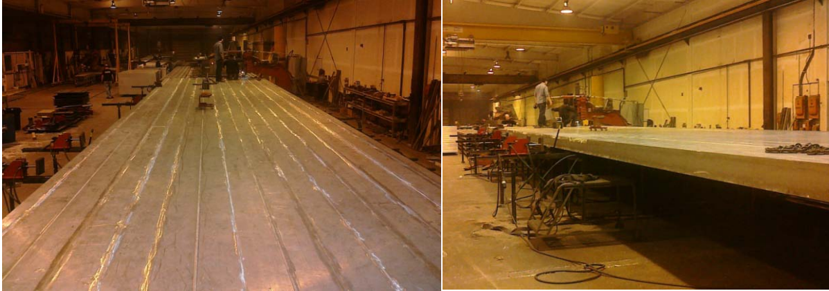
Aluminum bridge deck being Friction Stir Welded together.
