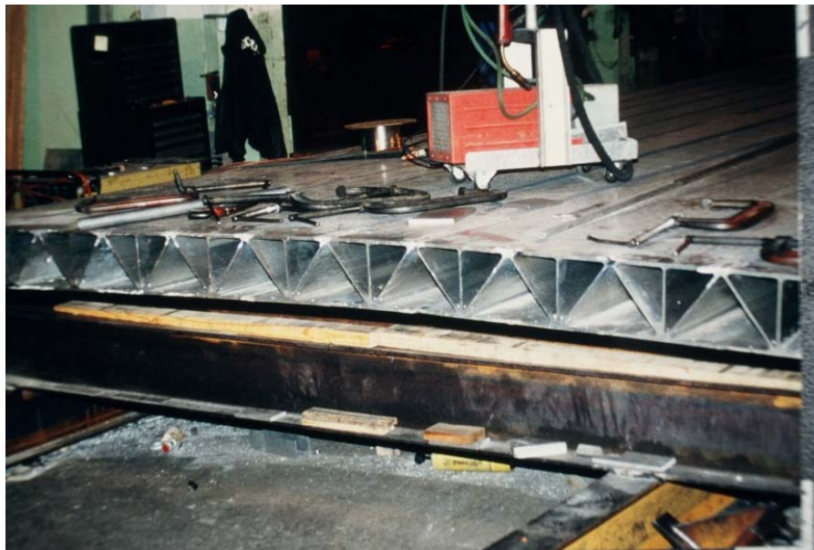
Arc welded deck being fabricated in late 1996
