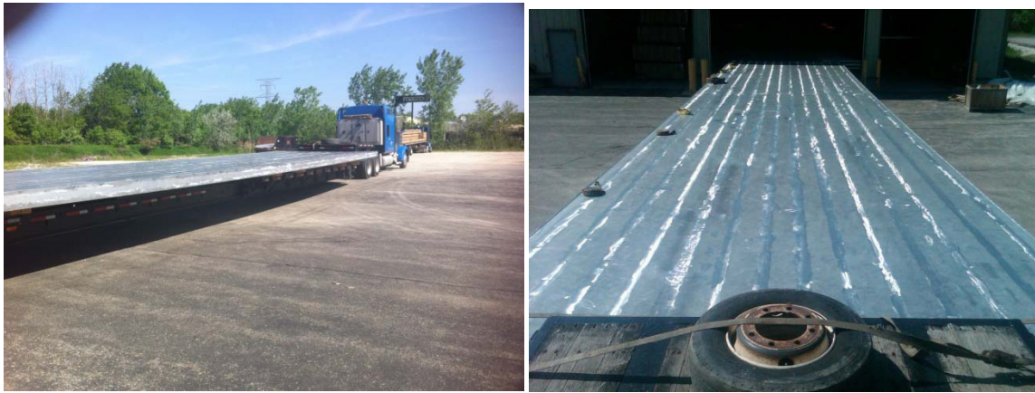
Aluminum bridge deck after fabrication using Friction Stir Welding
