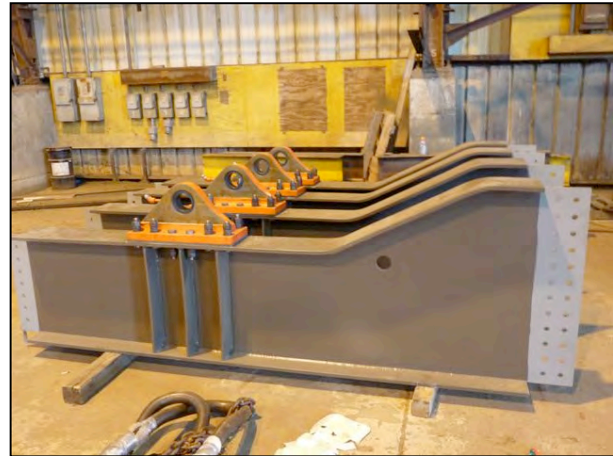
Photograph: Clevis Brackets Mounted to Cylinder Girder in Shop
