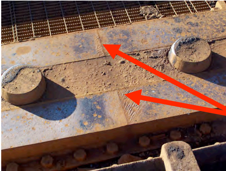
Photo No. 9: Looking south at north flat track. Note: plastic flow pattern at the joint in the casting
