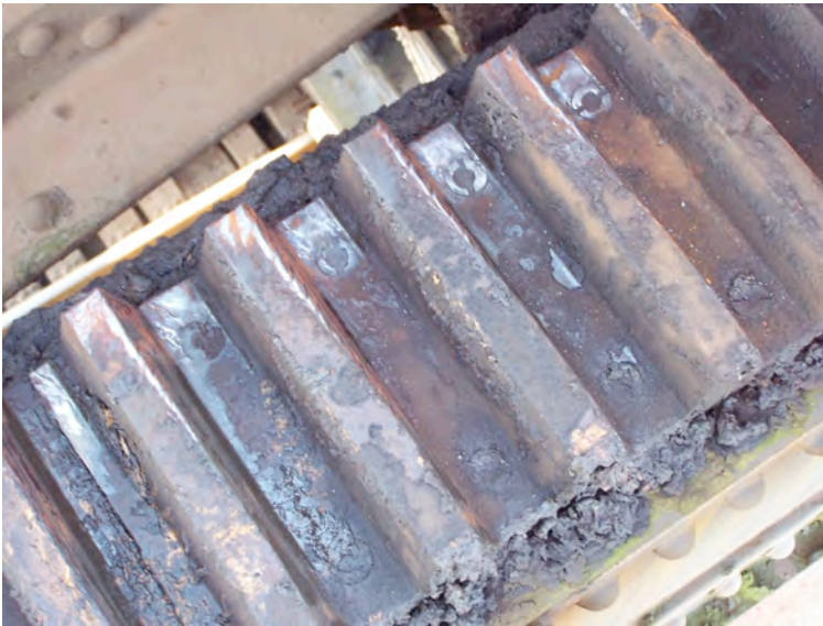
Photo No. 16: South rack/pinion interference at gear tooth 13 through 20. Note: severe binding between pack and pinion during opening, and damage to countersunk bolt heads
