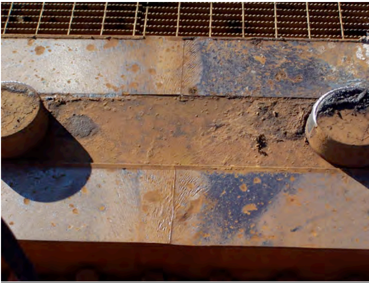
Photo No. 10: Looking north at south flat track. Note: plastic flow pattern.
