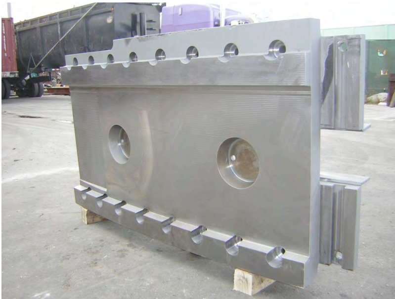
Photo No. 25: View of bottom of tread plate segment. Note circular sockets to match existing pintles, interlocking tongue and groove connections between the segments. Also note that the locations of the holes for bolted connections to flange angles are different on the two sides of the tread plate.
