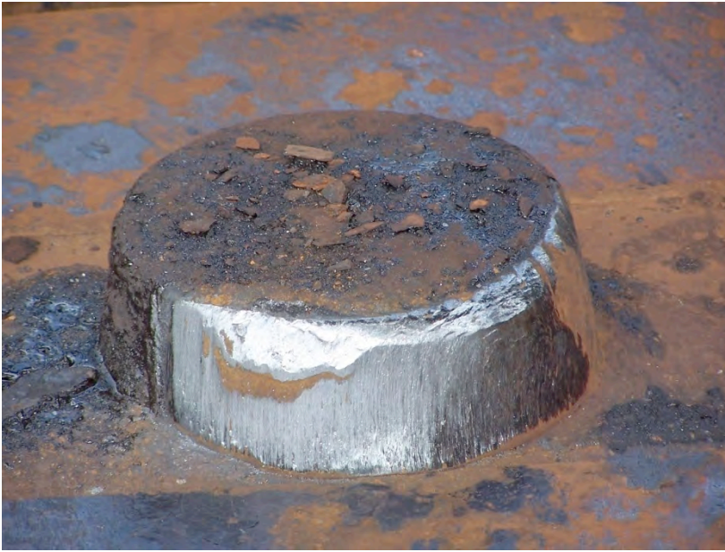
Photo No. 4: Close up view of Pintle. Note extensive plastic flow.
