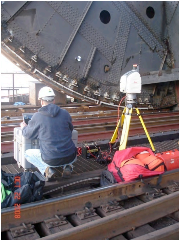
Photo No. 20: Laser survey of the segmental girders.
