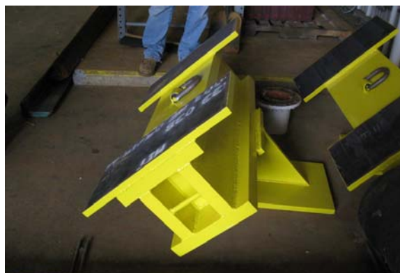
Figure 6 – Chock beam assembly in the shop
