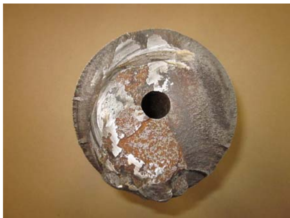
Figure 3 - Fatigue crack through the inboard face of the north counterweight trunnion pin
