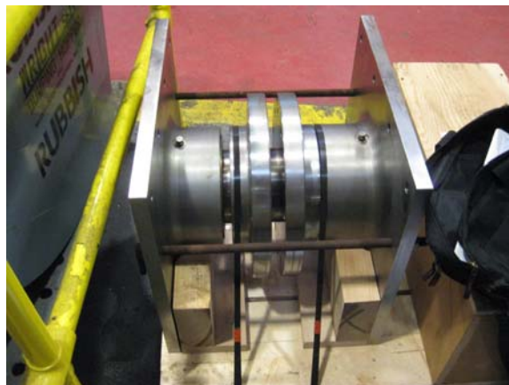
Figure 11 – Assembled counterweight trunnion in the shop
