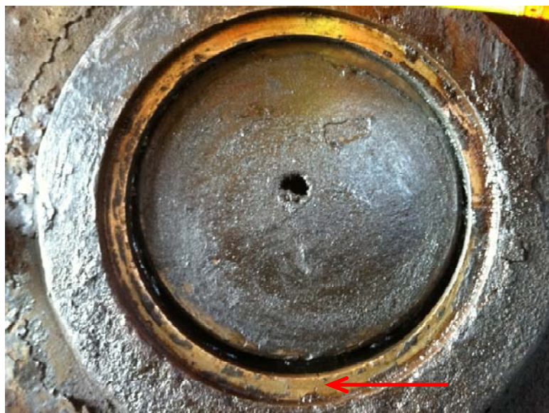
Figure 24 – The center counterweight trunnion bushings were cracked and had excessive clearances
