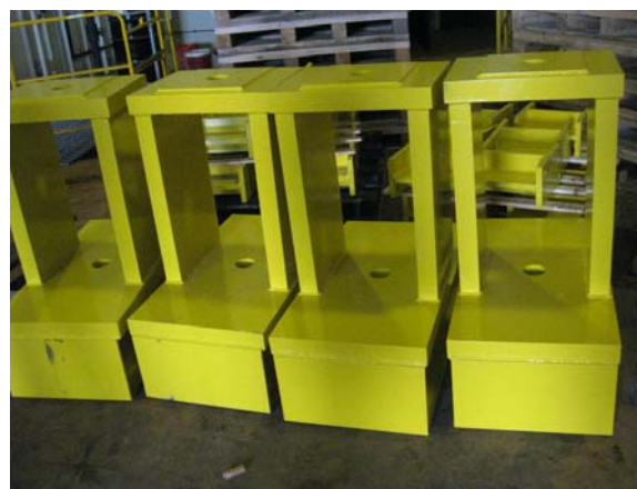
Figure 8 – Jacking seats in the shop
