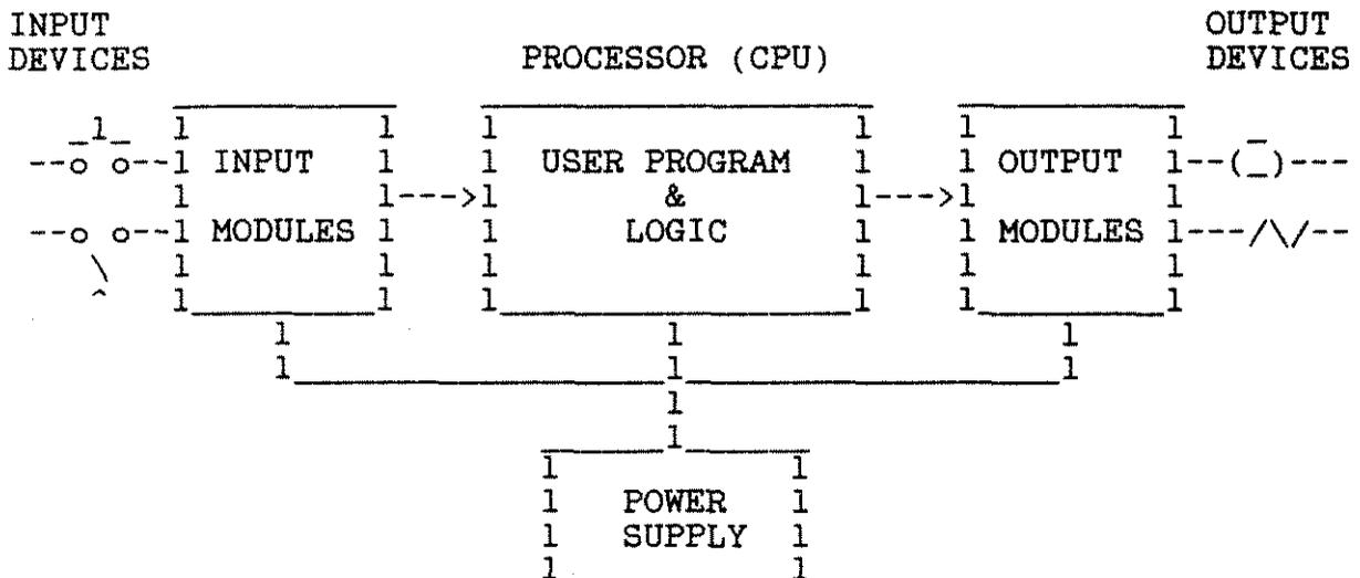
The left section is the input section. PC's must receive signals from various input devices to allow the PC to know what is going on in the real world. These inputs may be push buttons similar to the ones used to activate the bridge oncoming and offgoing gates and the traffic signals. They could be limit switches to indicate bridge or gate position, or they could be photo cells to indicate people or automobile presence on the bridge in critical positions.
