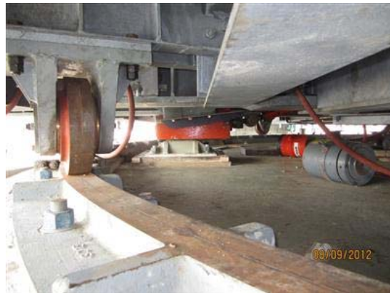
Photo 5: Redesigned Balance Wheel
