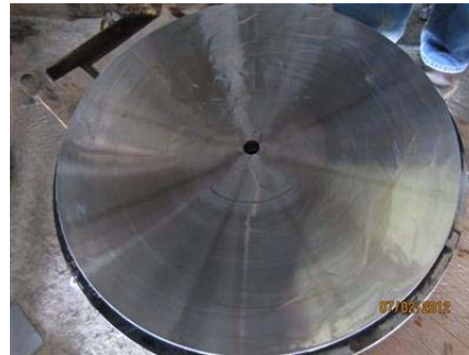
Photo 4: New Center Bearing Lower Steel Disk
