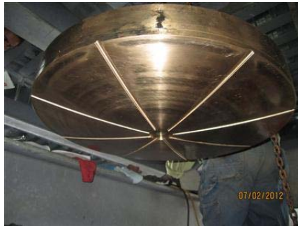
Photo 3: New Center Bearing Upper Bronze Disk
