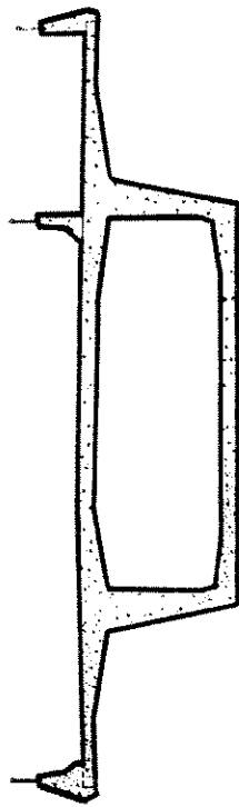
MAIN SPAN SECTION
