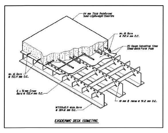
center in the upward facing web of a WT  $155 \times 10.5$  to provide a shear transfer mechanism between the concrete and steel.
