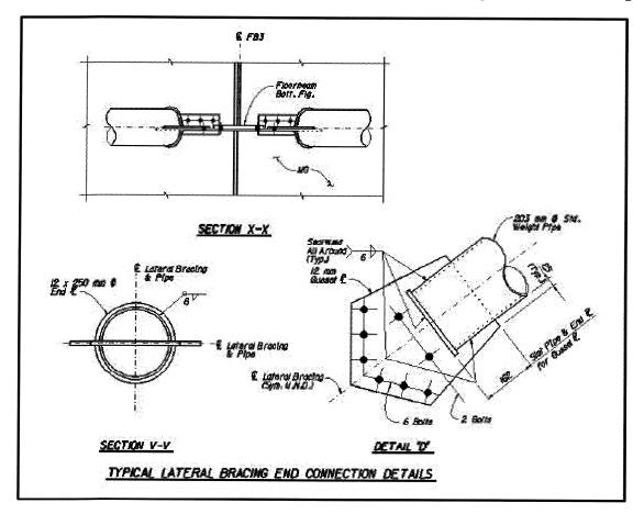
avoid these conditions and to utilize the lightest structural members practical for the bracing, pipe sections were used. Pipe sections do not have a weak bending axis making them ideal for bracing
