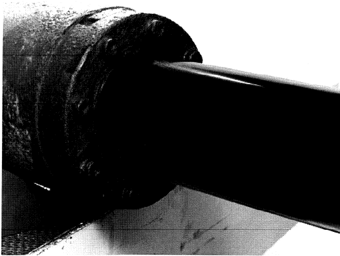
Fig. 1 : Hydraulic cylinder with CERAMAX coating
