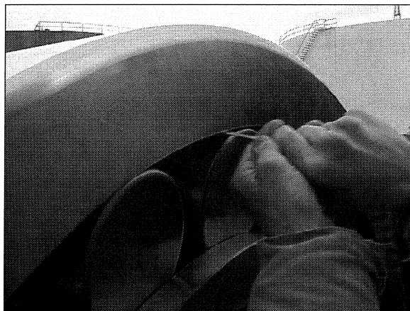
The bearing should be blocked while the RIC is measured at 12 o'clock.
