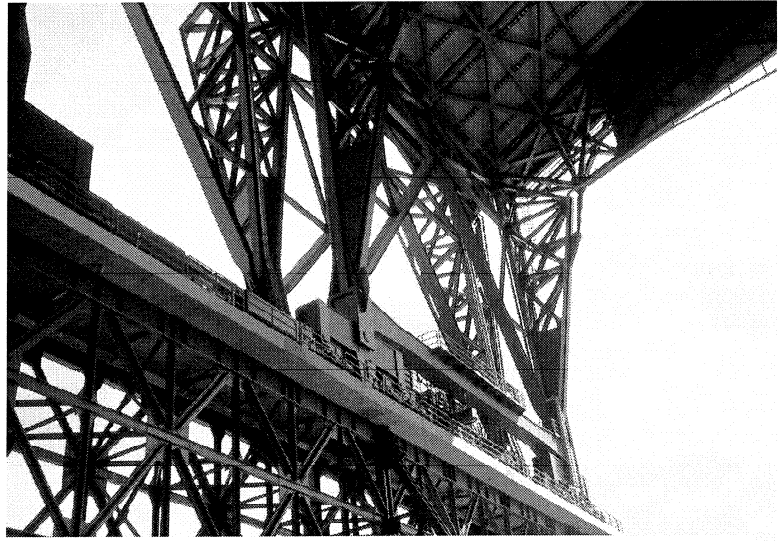
Figure 3 - Travel truck assemblies on top of elevated runways
