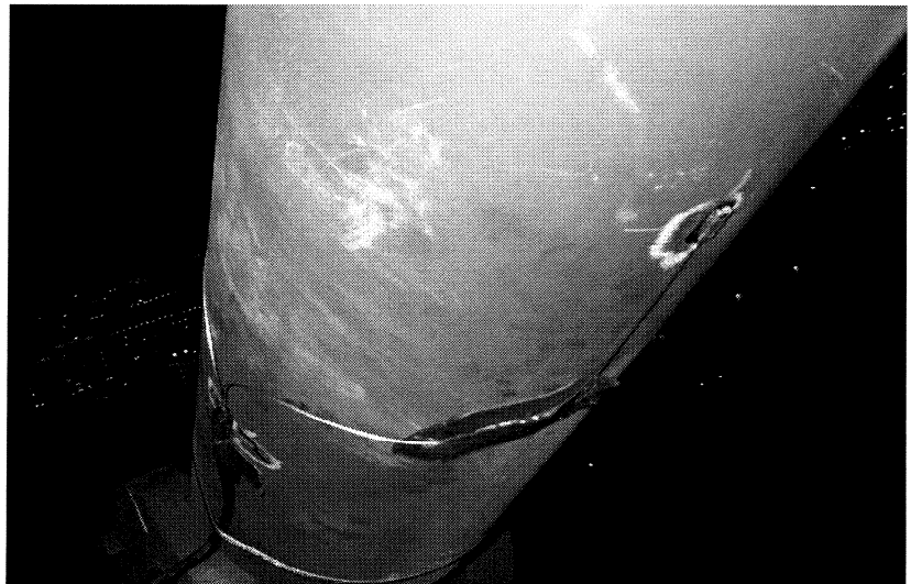
Figure 7 - Strain gages spot-welded on damper strut
