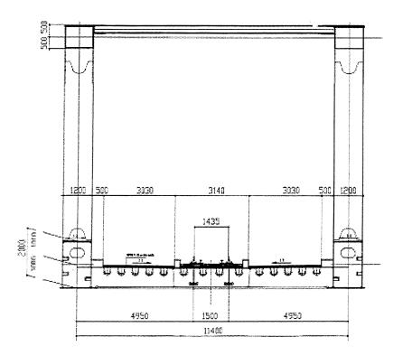
Figure 2: Cross Section Road Deck (Ref. 6)
