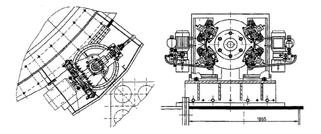
Figure 6: Top View of Drive With Brakes (Ref. 3)
