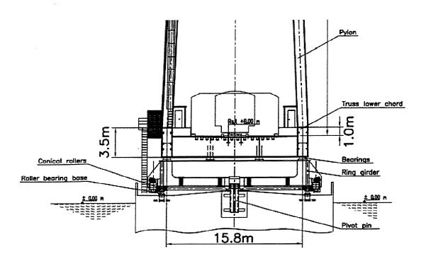
Figure 3: Cross Section at Pylon (Ref. 6)
