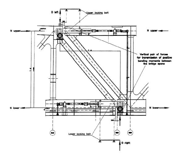
Figure 7: Longitudinal Section of the Centre Locking System (Ref. 6)
