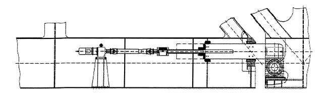
Figure 9: Detail of Bridge Centre Locking (Ref. 7)
