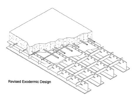
Research conducted at Clarkson University confirmed the viability of this approach, and included pull out tests, beam tests, full scale panel tests to ultimate, and a full scale, two span continuous fatigue test.
