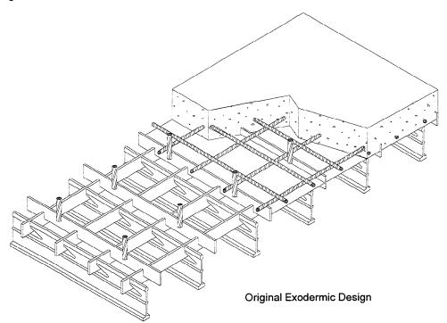
With this design, the neutral axis is located near the top of the grid, reducing the stress range at the fatigue prone welds and punchouts inevitable in a fabricated steel grating. Fatigue should always be checked in these type of decks, but rarely will control in an Exodermic design.
