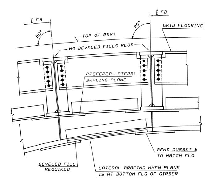
WHEN THE FLOORBEAMS ARE SET NORMAL TO GRADE, BEVELED BILLS CAN BE ELIMINATED. THIS ALSO APPLIES TO THE LATERAL BRACING PLANES WHEN THE BRACING PLANE IS LOCATED AT THE BOTTOM FLANGE OF THE FLOORBEAMS.
