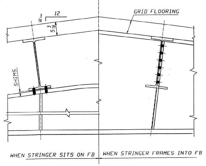
WHEN BASCULE SPAN HAS A CROSS SLOPE
