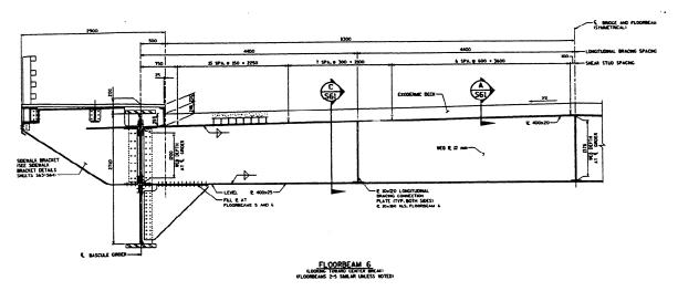
Framing consists of floorbeams at 4.1 meter spacing, with longitudinal and bottom lateral bracing. In the absence of stringers, the exodermic deck spans floorbeam to floorbeam. The exodermic deck will be composite with the floorbeams through the use of standard welded headed shear studs.
