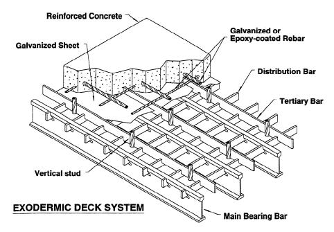
Exodermic decks are made composite with the steel superstructure by using headed studs welded to stringers, floor beams, and main girders as appropriate, and embedding these headed studs in a concrete haunch area. The haunch area is poured at the same time as the reinforced concrete deck where the deck is cast-in-place, or separately with a pre-cast deck. Exodermic decks require no field welding other than that required for the placement (with an automatic tool) of the headed shear studs.
