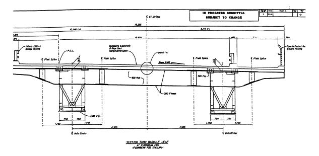
Main girders are steel boxes. Floorbeams are at 4.4 meter spacing. Cantilevered brackets (floorbeam extensions) extend 2.875 meters beyond the outside edge of the box girders. In the absence of stringers, the exodermic deck spans floorbeam to floorbeam. The exodermic deck will be composite with both the floorbeams and the top flanges of the box girders.
