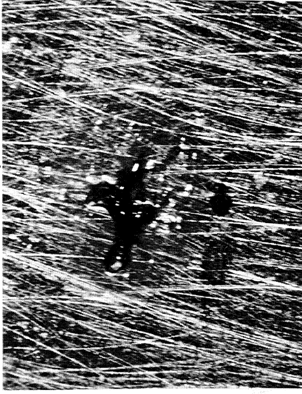
Stage A Fretting Wear After 6000 Cycles, With Grease Present, Contaminated With Black Wear Fragments
