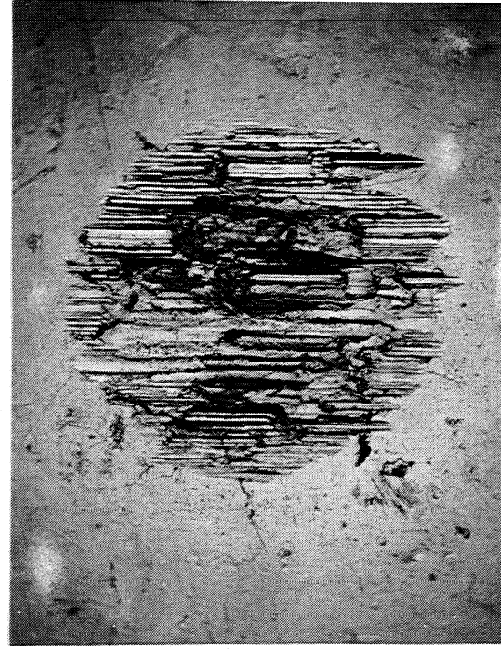
Figure 5. Micrographs of Wear Scars After Fretting Wear With Mineral Oil/ Polyurea Gelling Agent Grease.
