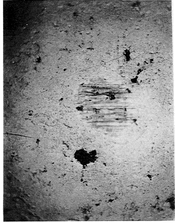
Grease Removed Revealing Wear Scars
