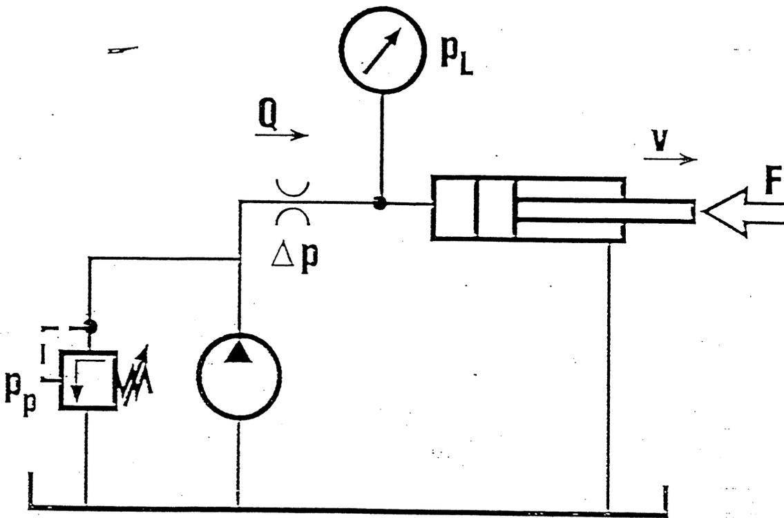
Fig. 1: Basic principle of the throttle control system
