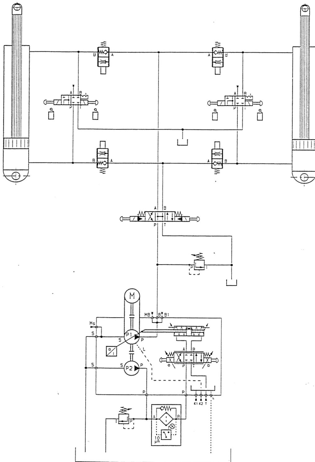
Fig. 6: Block diagram of hydraulic system
