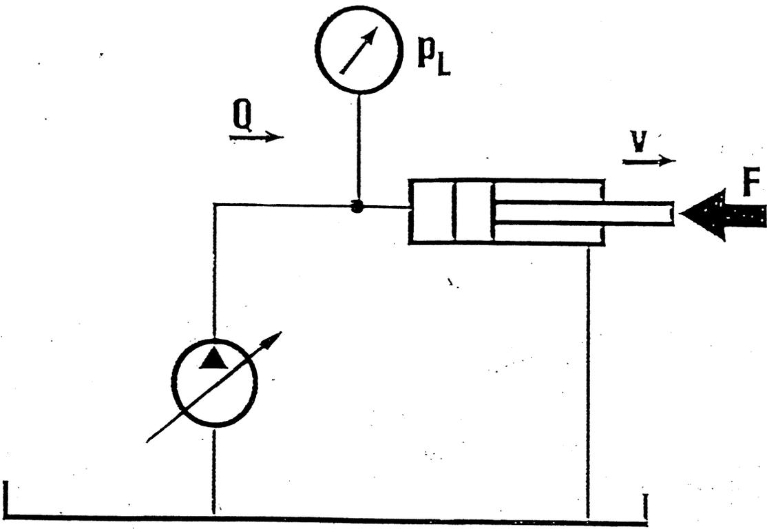
Fig. 3 : Basic principle of a pump control system
