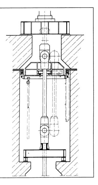
Due to shipping and assembly requirements the body comes in three parts; the individual parts of the sluice gate are screwed together.
