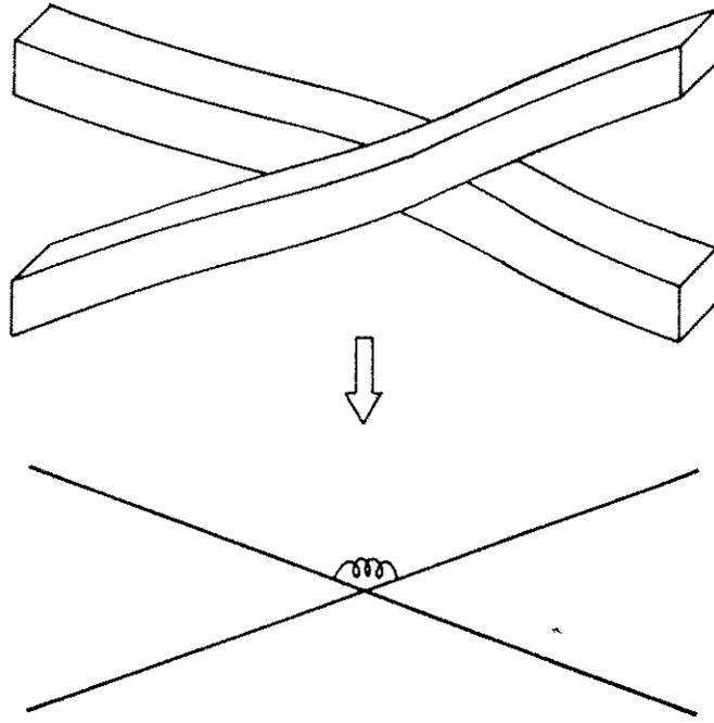
Figure 18: Friction Mechanism and Equivalent Model
