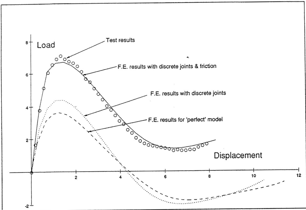
Figure 19: Load-Displacement Curves for a Curved Pentagonal Unit
