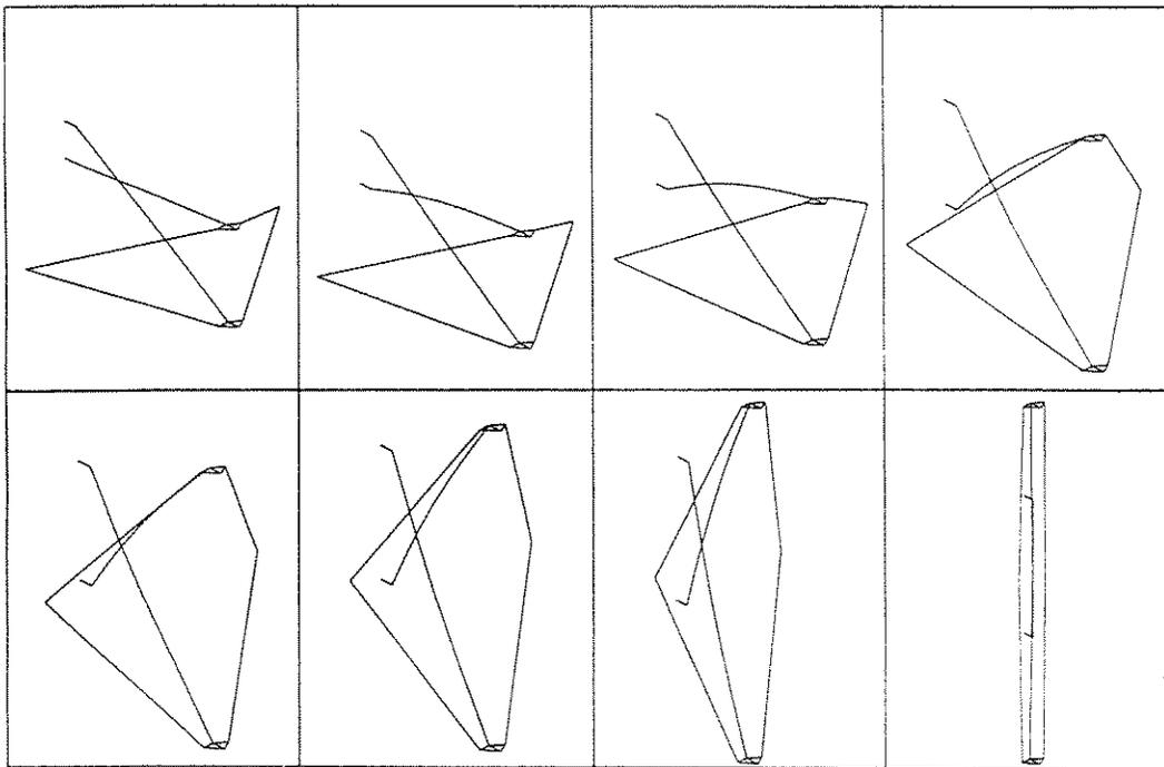
Figure 15: Successive Deformed Configurations of Discrete Joint Mesh
