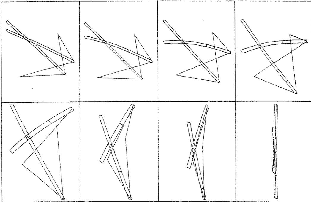
Figure 10: Successive Deformed Configurations of the Shell Mesh
