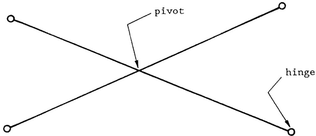
Figure 2: A Typical Scissor Like Element
