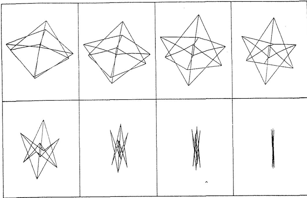
Figure 6: Successive Deformed Configurations from Deployment to Collapse
