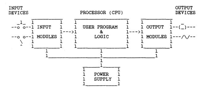
The left section is the input section. PC's must receive signals from various input devices to allow the PC to know what is going on in the real world. These inputs may be push buttons similiar to the ones used to activate the bridge oncoming and offgoing gates and the traffic signals. They could be limit switches to indicate bridge or gate position, or they could be photo cells to indicate people or automobile presence on the bridge in critical positions.
