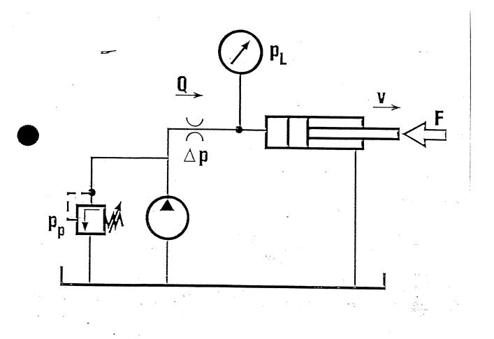
Fig. 1: Basic principle of the throttle control system
