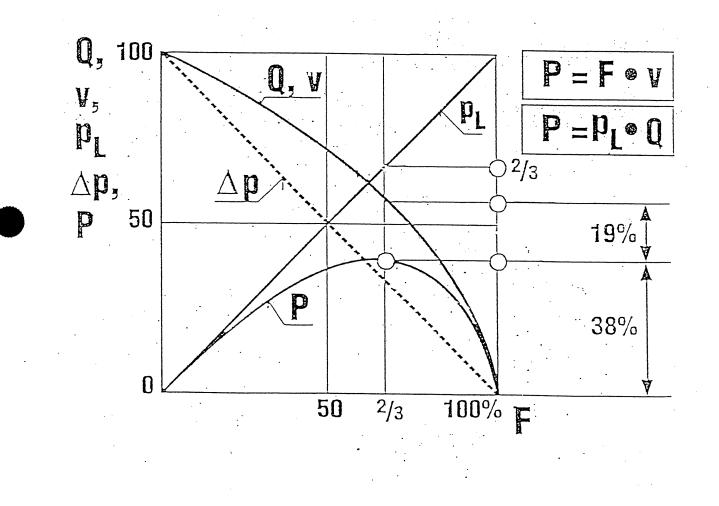
Fig. 2 : Performance potential of the throttle control system
