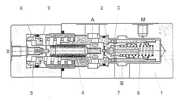
Fig. 8 : cross section of a check Q-meter
