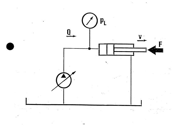
Fig. 3 : Basic principle of a pump control system
